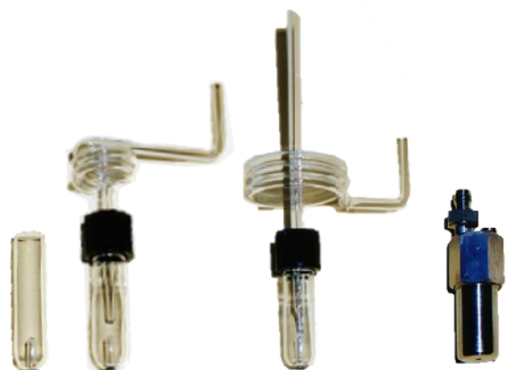
Pic 2: RADEX Glass open / Inert gas evolution / Autoclave
