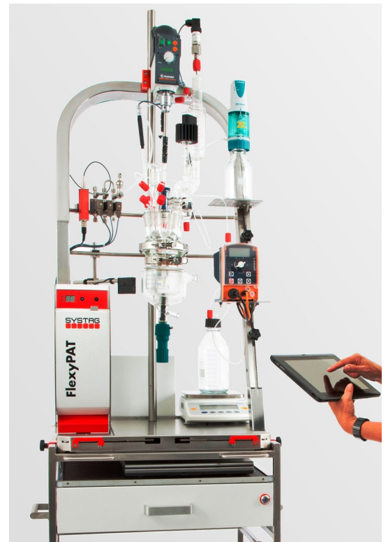
Operation using a tablet (Wi-Fi)
